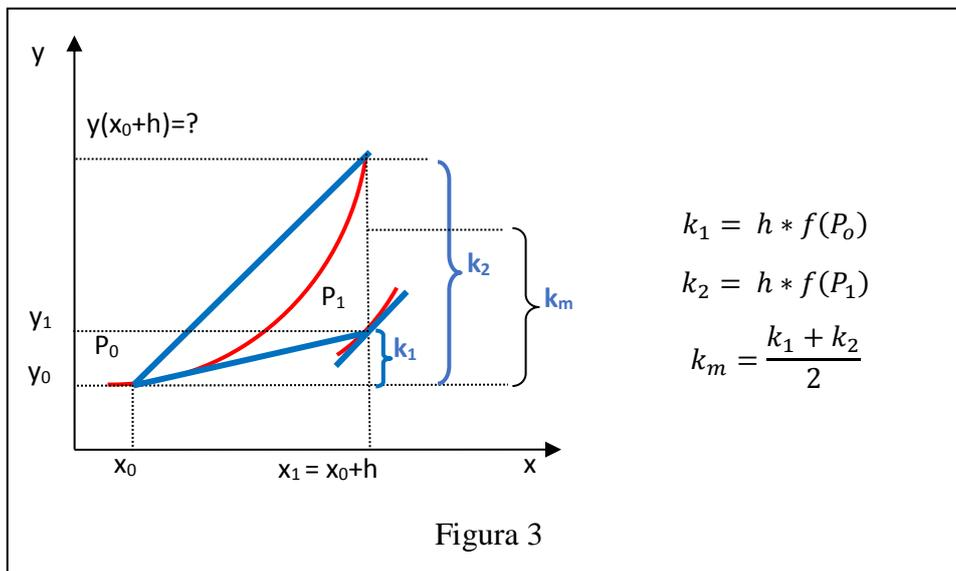
$$y_1 = y_0 + \underbrace{h * f(P_0)}_{k_1} \quad \text{con } P_0(x_0, y_0) \quad \text{determino} \quad P_1(x_0 + h, y_1)$$
